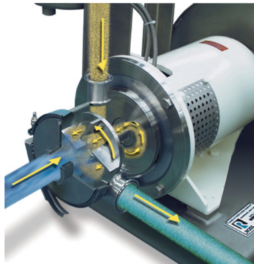
Example of an inline (continuous) powder injection system. The liquid stream (blue) enters the mixer and immediately encounters the powder addition (yellow). The resulting dispersion (green) is expelled from the stator openings at high velocity.
