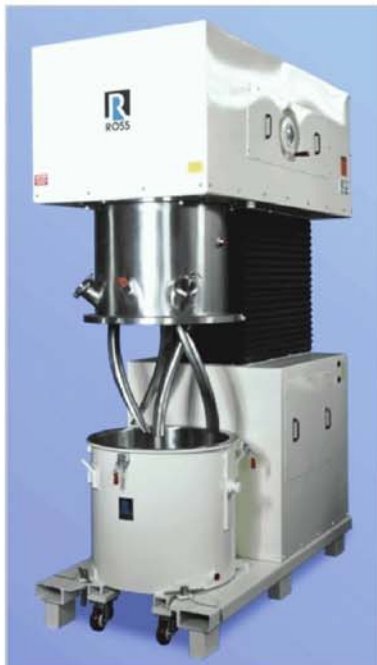
Figure 3. Ross Double Planetary Mixers equipped with High Viscosity "HV" Blades (U.S. Patent No. 6,652,137) are capable of handling very dense or thick applications up to around 6 million centipoise.
