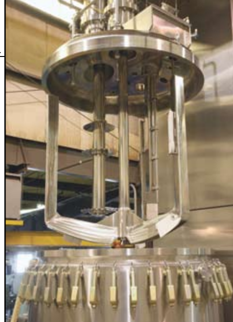
FIGURE 1. A two-wing anchor agitator is a cost-efficient answer to limited flow within a mix vessel. For batches up to approximately 200,000 cP, the anchor can generate significant flow, accelerate the dispersion and hasten progress toward batch uniformity
