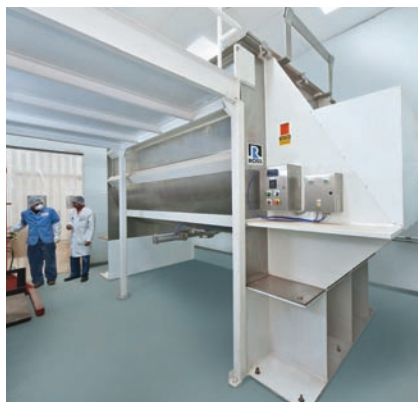
This 385-cu-ft sanitary ribbon blender currently processes green food powders, along with chocolate and red berry powders, in long production runs. Downstream from the blender, Bactolac ships these products in a wide variety of packages, from 30-gal drums to jars, bottles, and pouches.
